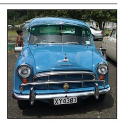
Graeme has been a very big help as he sandblasted all the clips for me and cut new gasket rubbers for under the chrome parts. I sandblasted the boot, bonnet and mudguards. Graeme fixed the rust in the guards for me. I also changed the 1500cc motor for a Morris Marina 1800cc engine.
