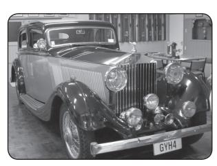
The 20-25 hp, introduced in 1929, was a development of the "small" owner-driver 20 hp of 1922-29 and was followed by the 25-30 hp and then the Wraith in 1938. All had overhead valve 6 cylinder engines starting at 3127cc and growing to 4257cc. Compare those sizes with those of the 40-50 hp (7428cc from 1909), the 1925 Phantom I and 1929 Phantom II (7668cc), and the V12 Phantom III of 1937 (7338cc!)
